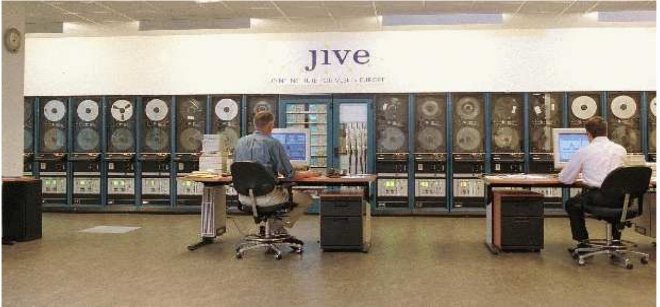
Figure 3. The EVN correlator at JIVE has been operational since the end of 1999. This picture shows the setup with all 16 station inputs from tape units. Currently half the inputs are disk based recorders. The PCInt project will enable the EVN correlator to generate and handle output data rates as high as 160 MB/s or 13 TB/day. This will permit the full capacity of the correlator to be harnessed.
