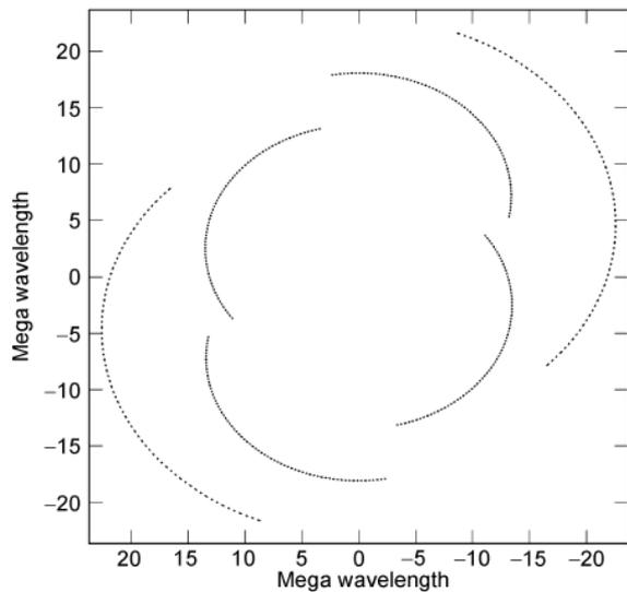
**Figure 1** The  $(u, v)$  coverage obtained for PSR B0329+54 at 2.2 GHz from 3 baselines formed from the CVN antennas Shanghai Kunming and Urumqi.
