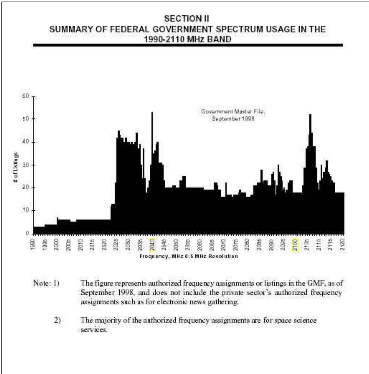
Fig. 5-1. Frequency allocation regime in according to the US Federal Regulations [5].
