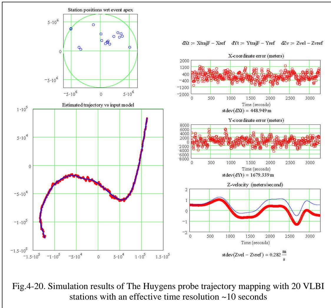
Smoothing the XY data over 100 s with a Gaussian window yields RMS errors for the trajectory estimate of 260 m and 970 m for X and Y coordinates respectively.
