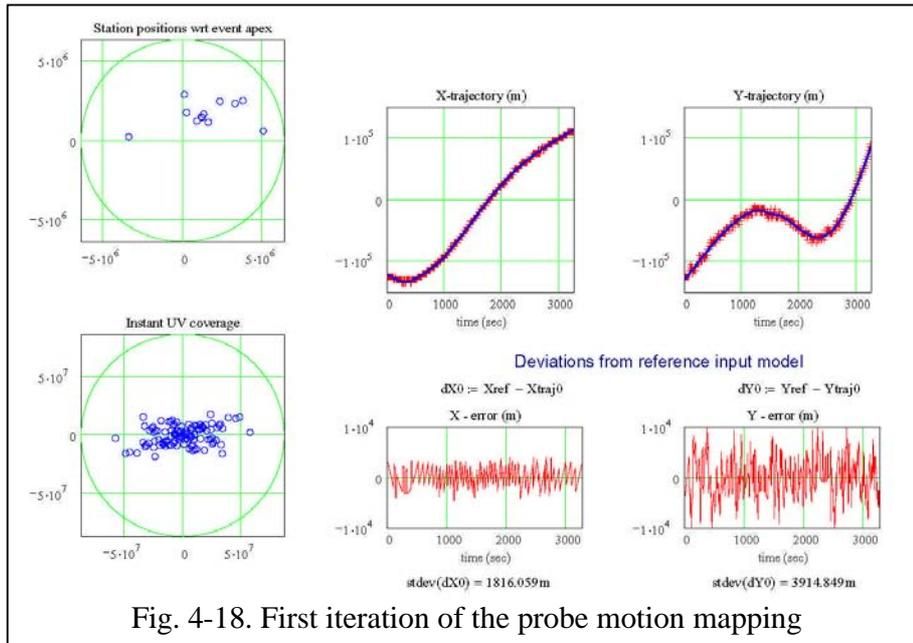
After upgrading the probe motion model several times, including more distant telescopes, and improving the spatial resolution of the synthesized aperture, the final set of XY corrections for the probe position can be estimated.
