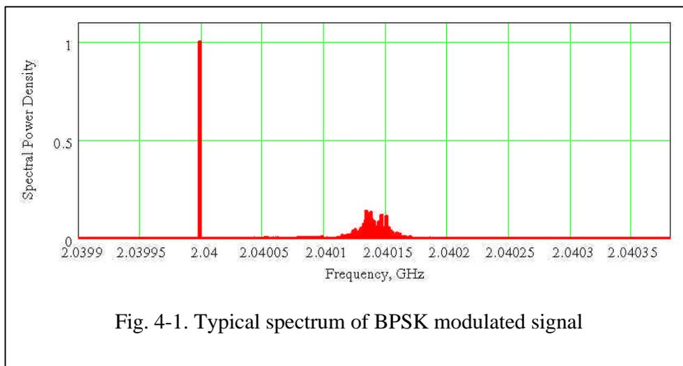
Fig. 4-1. Typical spectrum of BPSK modulated signal
