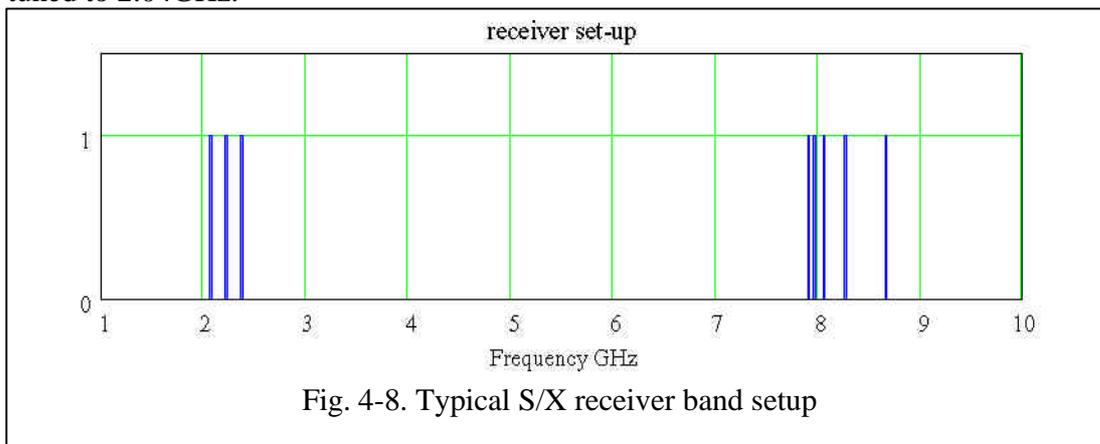
The total observed signal bandwidth for background radio sources can be as wide as 128 or even 256 MHz, split into 8 or 16 MHz wide sub-bands. By spanning a wide
