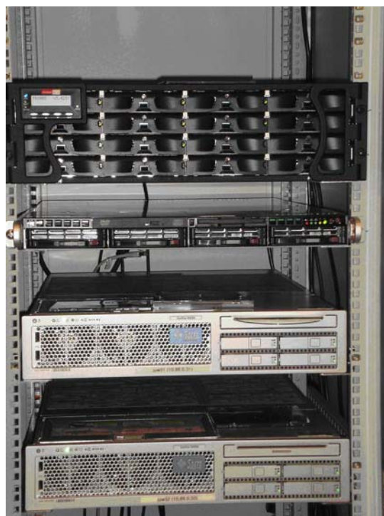
Figure 3.2: Software correlator platform (top) and new correlator control computers
