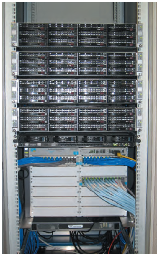
Figure 3.4: the SFXC cluster, consisting of four Transtec Calleo 642 servers. Each server contains four nodes, each node is equipped with two quadcore Intel Xeon 2.26 GHz E5520, giving a total of 128 cpu cores.
