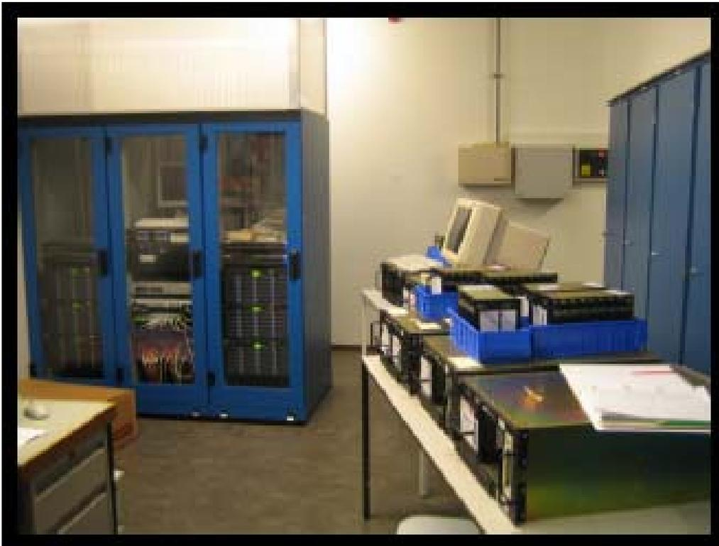
*Fig. 8.9.* Linux cluster used for narrow band Huygens VLBI processing. It consists of 6 dual core Opteron nodes equipped with 1.5 TB disk raids each interconnected via a FireWire switch and connected to Mark 5 VLBI recorders via optical 1GB Ethernet lines.
