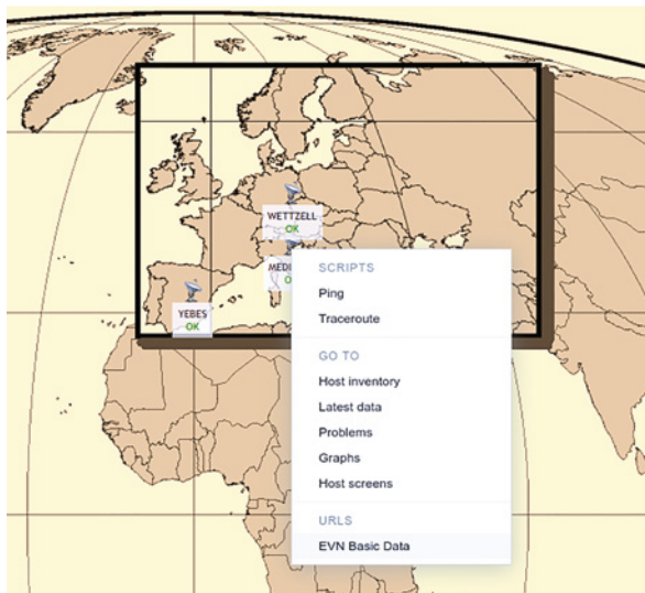
Figure 3.7: Two screenshots from the evn-monitor.jive.eu web interface. Left: welcome screen: showing stations who upload monitoring data into the system with right-click context menu. Right: an example of a time series kept in the central monitoring system: the Medicina DOT clock offset measurement over the previous week.
