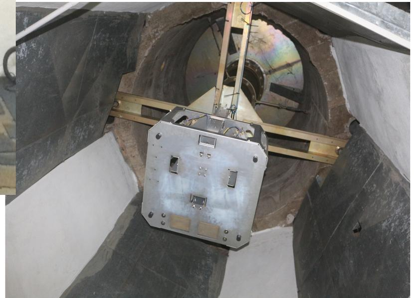
★ Dual Uncooled receiver (C-band) system at central frequencies of 5 GHz and 6.7 GHz
