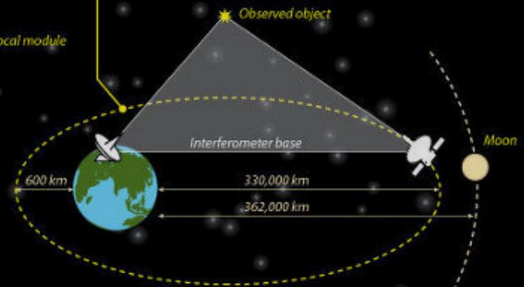
The RadioAstron observatory will operate with an international network of ground-based radio telescopes. This huge ground- and space-based telescope system, also called an interferometer, will provide the finest angular resolution.
