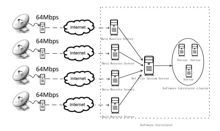
Data Flow Diagram in Chang'E 3 Mission based on e-VLBI technology
