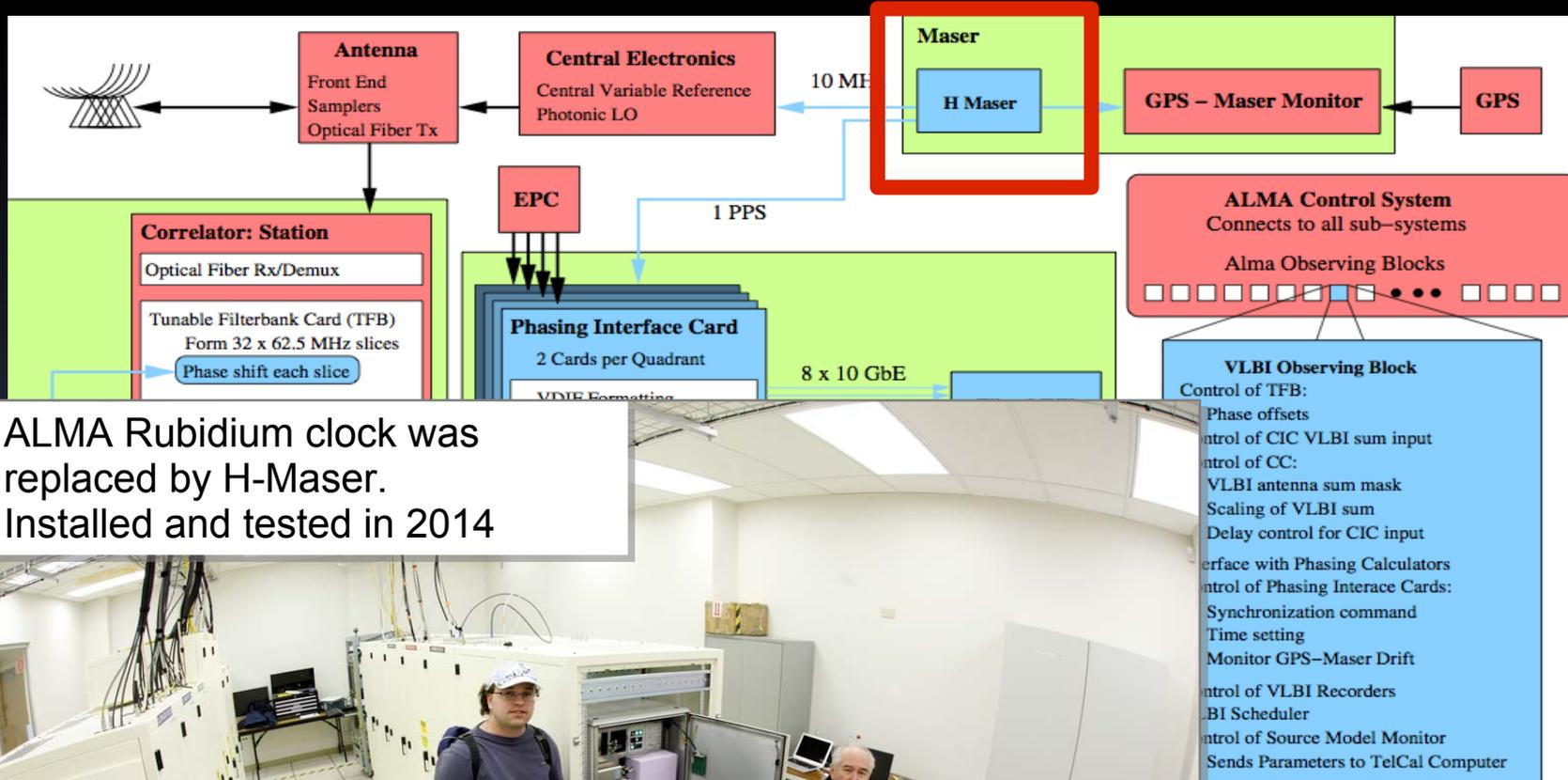
ALMA Rubidium clock was replaced by H-Maser. Installed and tested in 2014
