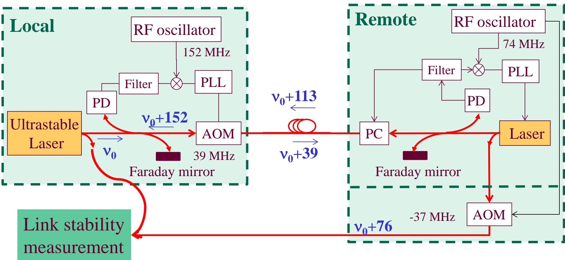
Autonomous lock (microcontroller), no stable RF clock at remote end, optical regeneration (PLL), automatic polarisation controller,
