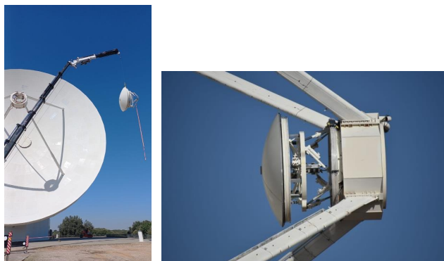
Figure 1: Wobbler system for RT40 (left: previous configuration, right: wobbler configuration with new hexapod to support load increase)
