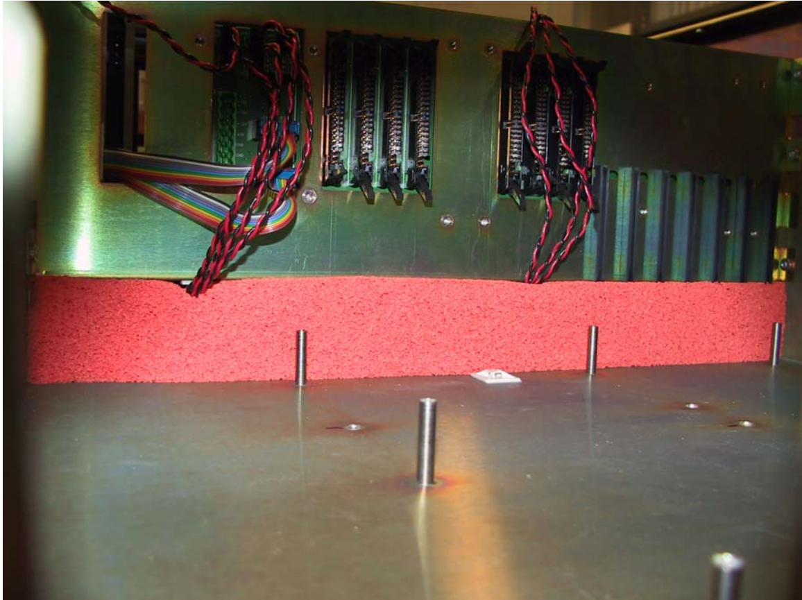
Picture 10: Rubber foam in place
