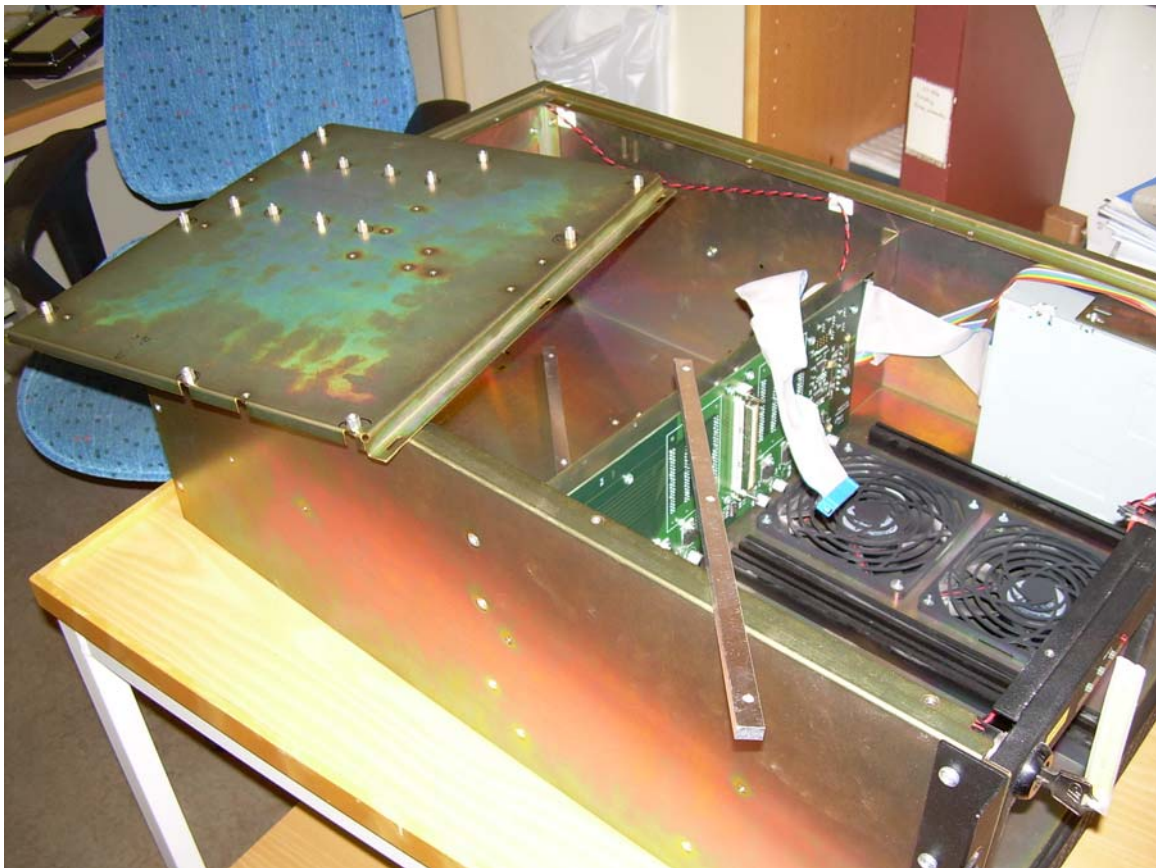
Picture 7: Metal base plate with standoffs for server board. Note the long aluminum rod in the foreground, used to fix the plate to the bottom of the case.
