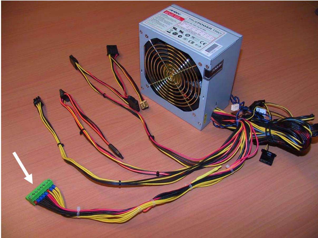
Picture 12: Power supply with backplane connector
