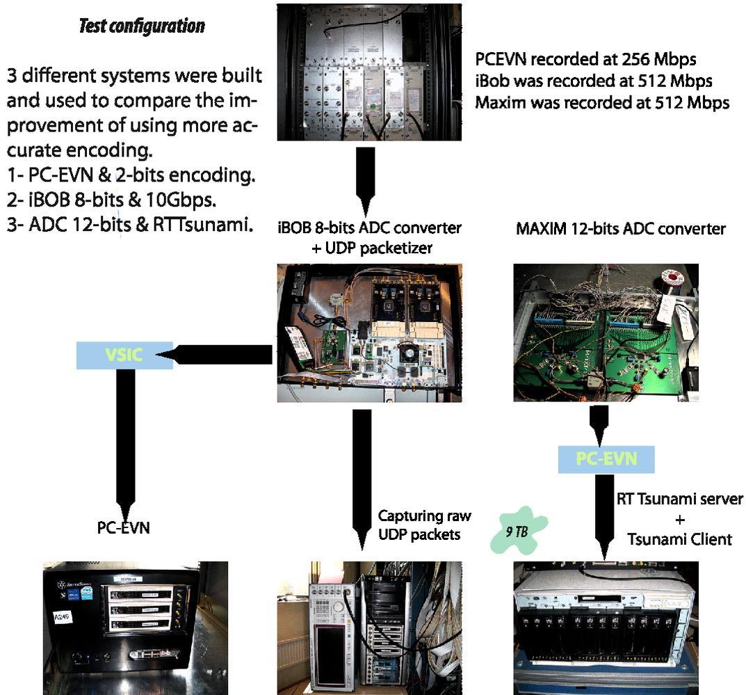
Figure 7: Configuration used for the latest tests, to record simultaneously using all three DASs.
