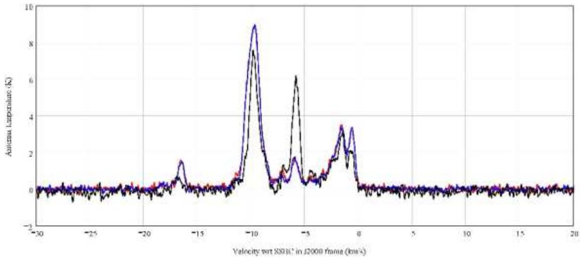
Figure 11: W75NB spectra during 06/02 (red), 06/03 (black) and 06/04 (blue) 2008. In the two first cases data was acquired with PC-EVN and for 06/04 iBOB (8-bits) was used.
