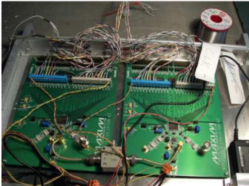
Figure 10: Building the enclosure to allocate both Maxim ADC samplers and the new wiring to convert the LVDS output mode to VSIB compatible.
