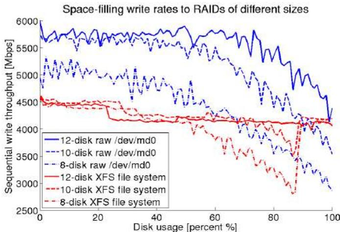
Figure 1: Space-filling write rates to RAID's of different sizes.
