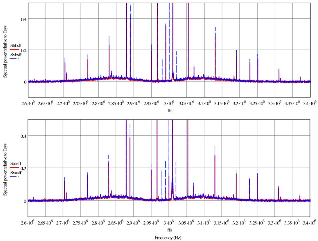
Figure 12: Upper image shows iBOB (red) and VSIB (blue) spectra and lower image shows Maxim (red) and VSIB (blue) data. S/C carrier signal is centered at 2.97 MHz and PCal is at 3.01 MHz.
