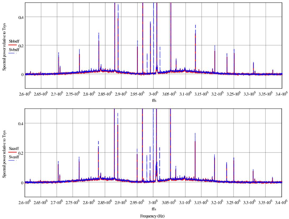
Figure 12: Upper image shows iBOB (red) and VSIB (blue) spectra and lower image shows Maxim (red) and VSIB (blue) data. S/C carrier signal is centered at 2.97 MHz and PCal is at 3.01 MHz.
