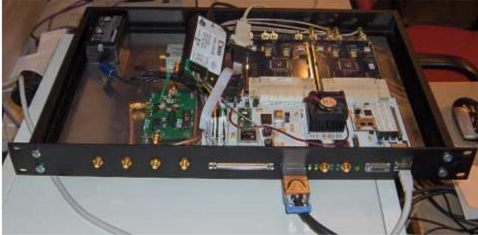
Figure 9: A current picture of the iBOB, two ADC sampler modules and the frequency synthesizer.
