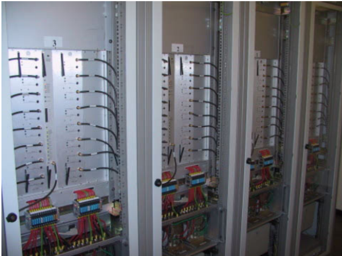
Figure S3: The heart of the EVN data processor at JIVE - a purpose-built super-computer developed to process VLBI data.
