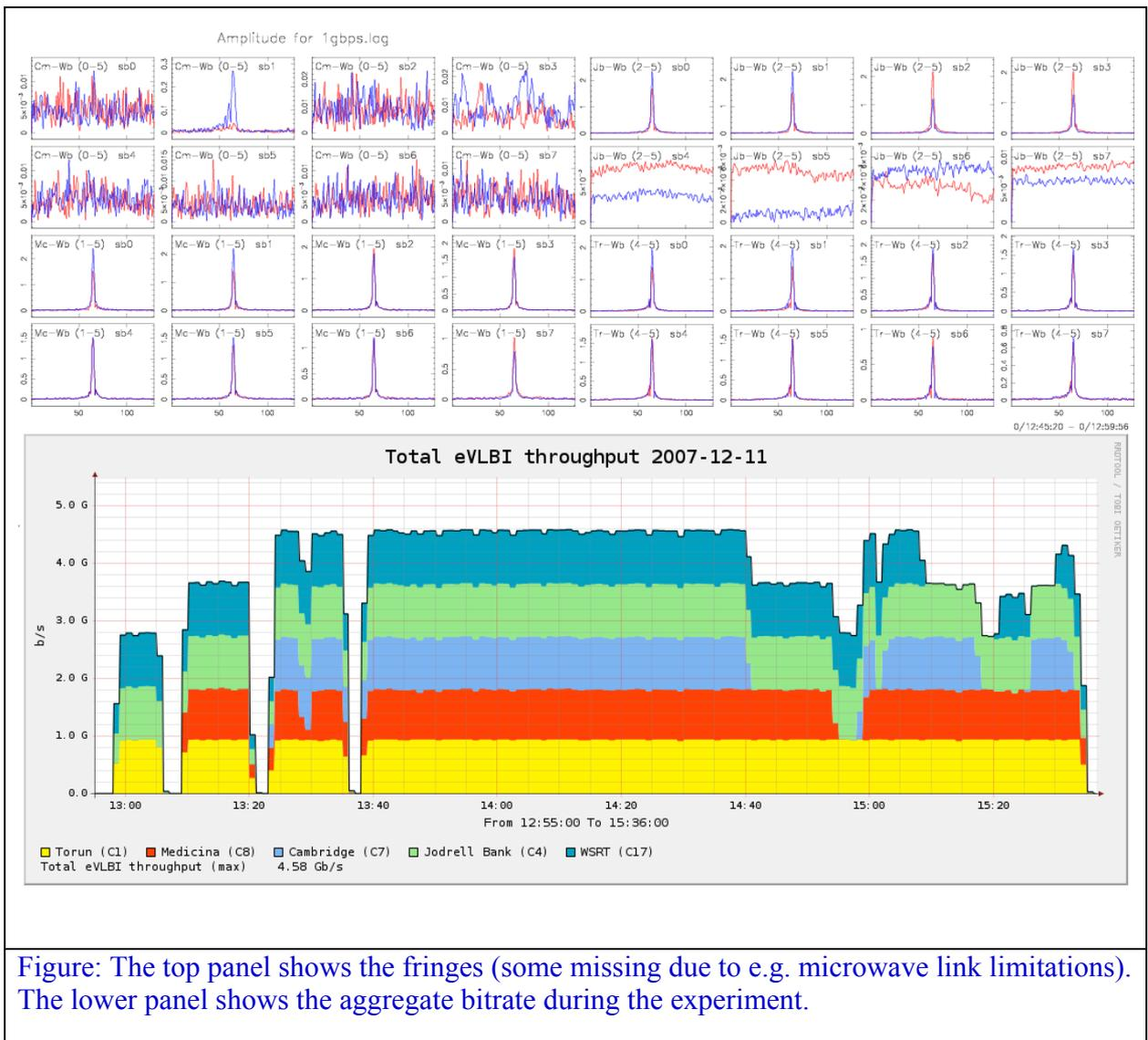
Figure: The top panel shows the fringes (some missing due to e.g. microwave link limitations). The lower panel shows the aggregate bitrate during the experiment.
