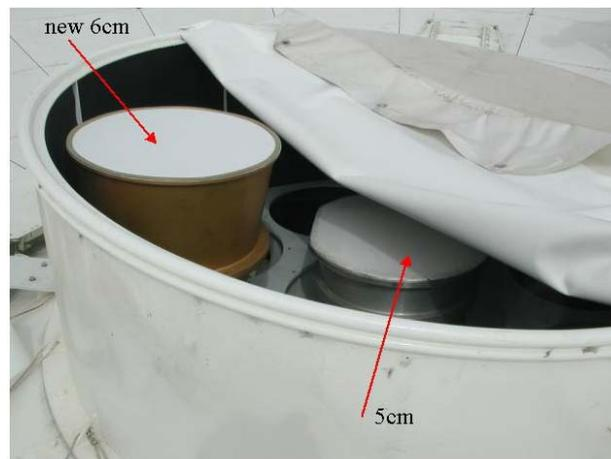
A new 6cm receiver has just been mounted on the VLBI parabolic antenna of the Medicina station, improving the sensitivity of almost a factor of two with respect to the old receiver..
