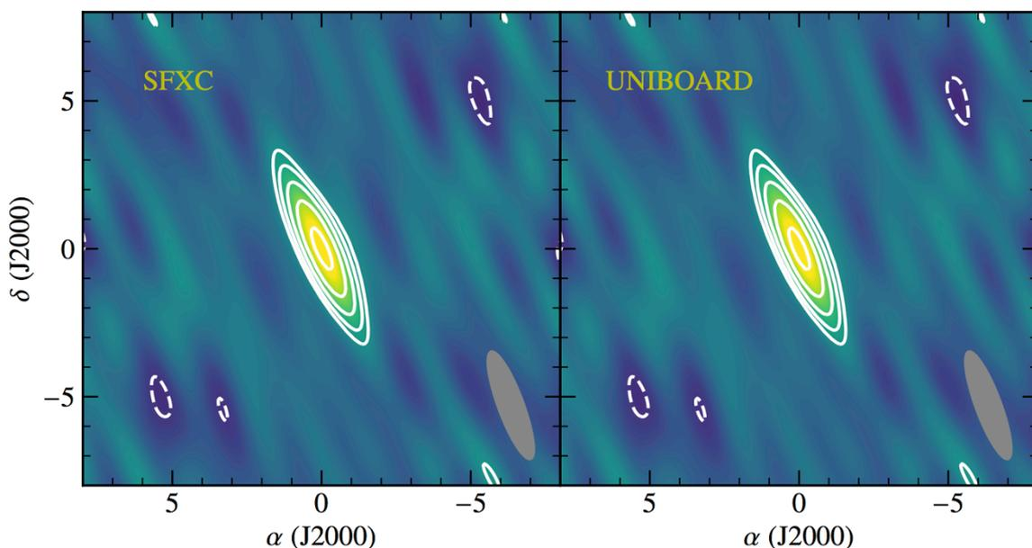
Figure 4: The final images obtained from this scan with the two correlations. It can be clearly seen that both images are identical, showing a compact source with a peak brightness of 5.16 mJy/beam and a noise rms level of 0.39 mJy/beam. The synthesized beam is  $3.9 \times 0.86$  mas, and contours start at 3 times the noise level with increments of square root of 2
