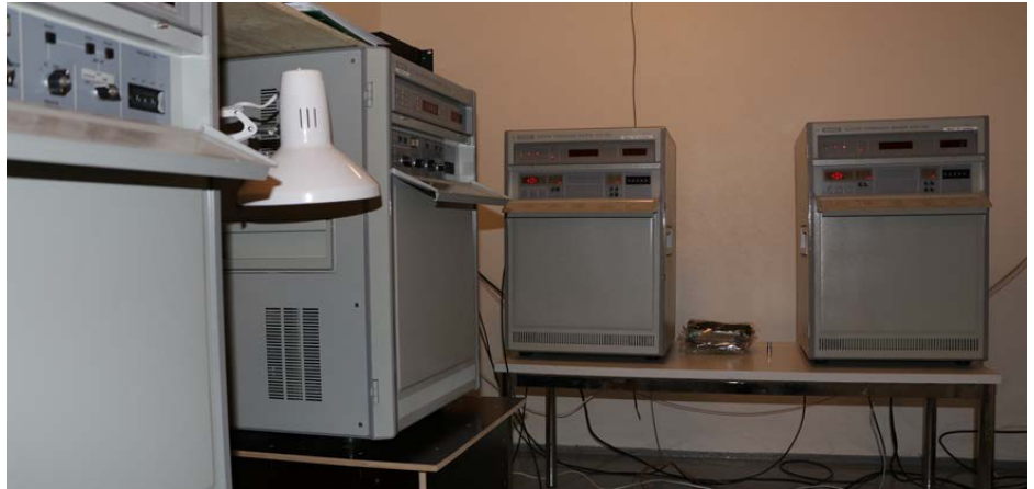
Figure 3. Metsähovi's four H-masers. On the left the old type CH1-75 masers, on the right the new type CH1-75A masers. The one on the far right, is now the house maser. Picture credit: Merja Tornikoski.
