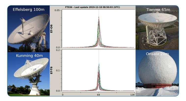
Fringes between the stations Effelsberg (Ef), Onsala (O6), and Tianma65 (T6) together with pictures of all stations involved in the test. Note that there are no fringes to Kunming due to a recorder failure at the station.
