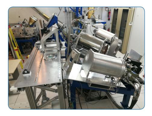
The high frequency receivers at the 40m RT receiver cabin. On the left, the hot and cold calibration system. The W band receiver is the one closer to the observer. The farther one is the Q band receiver and in between both, the K band one is located.
