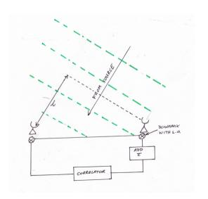
Coherence at antennas equals the absolute value of the normalized Fourier transform of the brightness distribution of the source. (Van Cittert-Zernike Theorem.) Geometric delay,  $\tau$  to align wavefronts is crucial!
