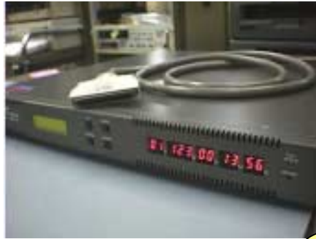
ADS1000 (1024Msample/sec 1ch 1bit or 2bits)
