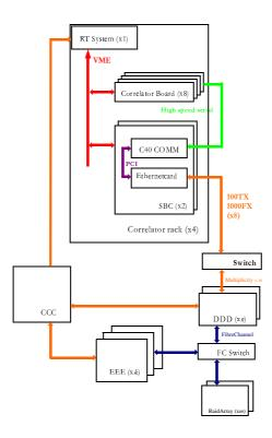
Figure 1: Schematic overview with all components installed
