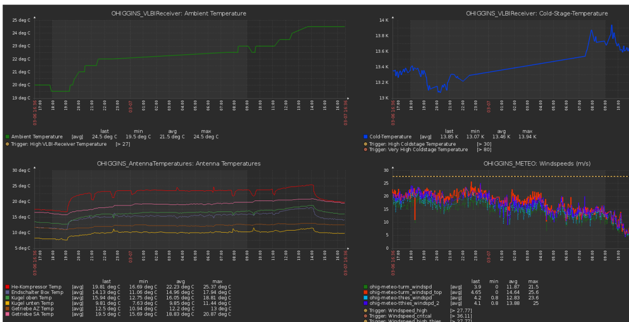
Figure 8. Test of data transfer of NASA Field System data via tunnelled HTTP connections and parallel tunnelled ZABBIX-Proxy connections for additional parameters over long-haul WAN connections with O’Higgins (Antarctica).
